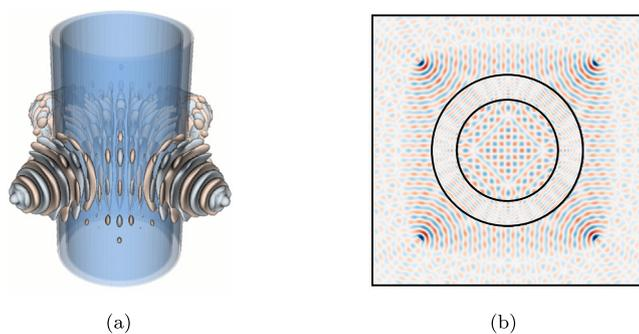
**Fig. 7.** Visualizations of four model humpback whales vocalizing towards an annular bubble net in (a) three- and (b) two-dimensions. The acoustics are shown via isocontours of pressure and the annular bubble net is shaded.
