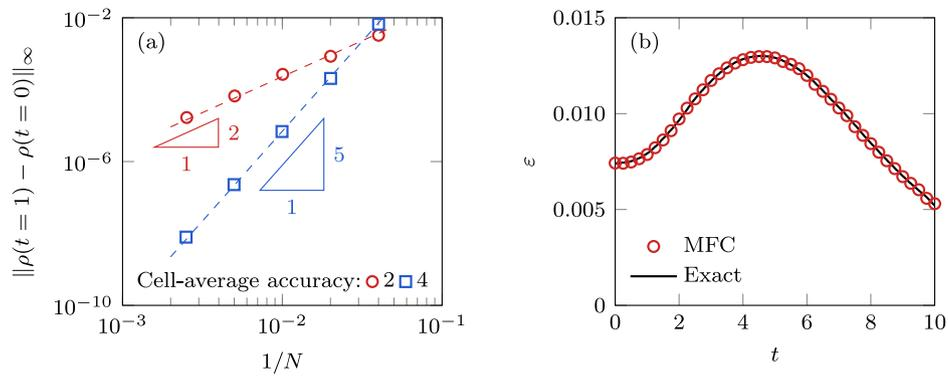
**Fig. 5.** (a)  $L_\infty$  density error associated with an isentropic steady vortex for the cell-averaged scheme accuracy labeled. (b) Non-dimensional kinetic energy dissipation rate  $\epsilon$  associated with the three-dimensional Taylor–Green vortex problem; the MFC solution is compared to the direct spectral solution of Brachet et al. [93].
