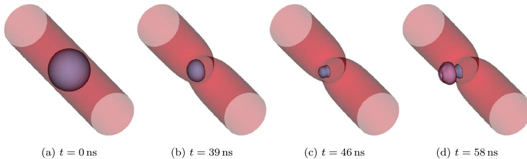
**Fig. 6.** Temporal snapshots (a)–(d) that show the bubble collapse and vessel wall deformation. The shock impinges the vessel from right to left. The bubble and vessel walls are illustrated via their 0.5 volume-fraction isosurfaces.
