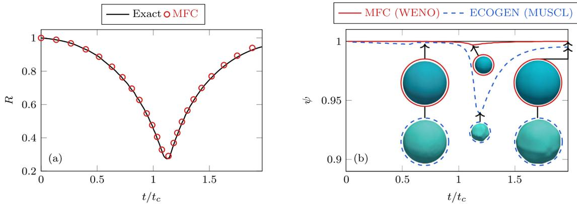
**Fig. 4.** Evolution of (a) the dimensionless bubble radius  $R$  and (b) its sphericity  $\psi$ . In (b) the nominal bubble shapes, represented by  $\alpha_l = 0.5$  isosurfaces, are shown at select times for MFC (WENO) and ECOGEN (MUSCL).
