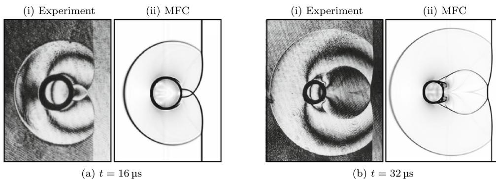
**Fig. 2.** Comparison between (i) holographic interferograms [88] and (ii) numerical schlieren visualizations using MFC at select times (a) and (b) as labeled. Source: The experimental images are reprinted from Igra and Takayama [88].
