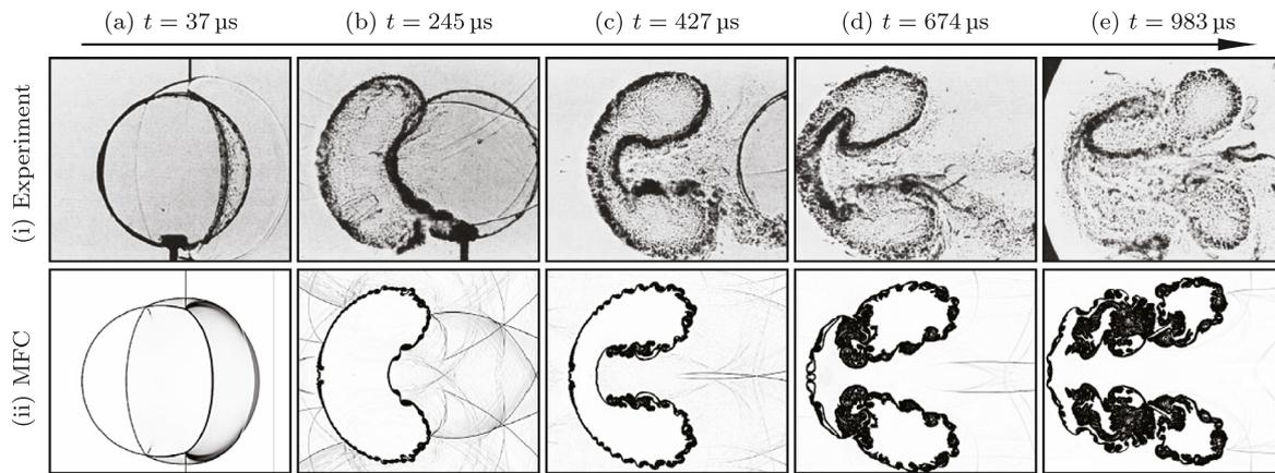
**Fig. 1.** Comparison between (i) experimental shadowgraphs of Haas and Sturtevant [81] and (ii) numerical schlieren visualizations [85] using MFC at select times (a)–(e) as labeled. Experimental images are ©Cambridge University Press 1987.
