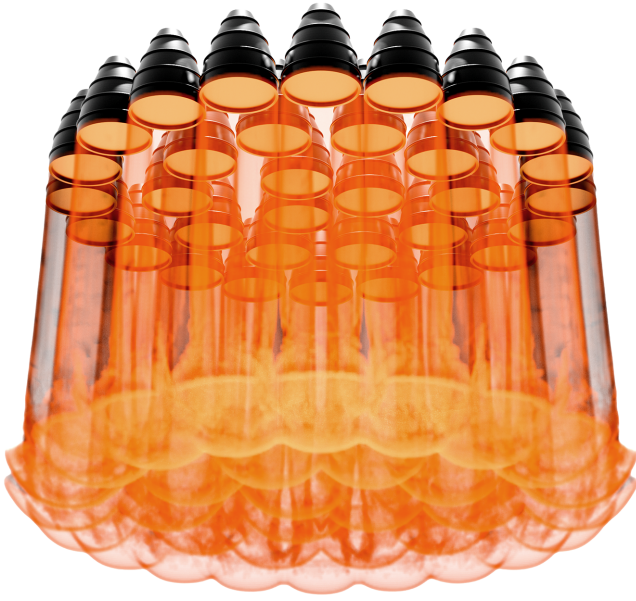
Figure 1: Simulation results showing the interacting plumes from an array of 33 thrusters in a configuration inspired by the SpaceX Super Heavy with 16.5 trillion degrees of freedom. (The thrusters themselves are for visualization purposes. We model them through inflow boundary conditions.)
