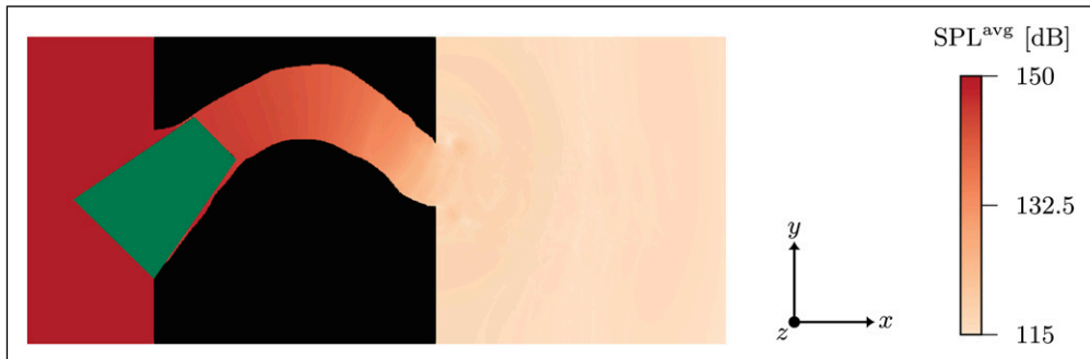
Figure 24. Time-averaged sound pressure level (SPL) distribution in the 2D x - y slice of the simulated 3D ear canal model with an ill-fitting earplug, subjected to a 1 kHz incident acoustic source at 150 dB.
